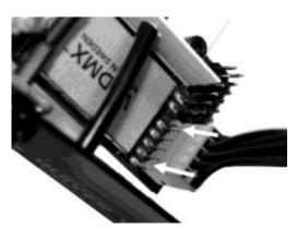
Re-assemble the PIVOTWDMX512 into the PIVOTC512 console using the same screws. Screw in and rotate the ANTENNA.
