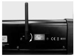
Turn ON the PIVOTC512 console and set the DMX universe for the wireless following the instructions on page 53 of console user → manual. The user manual file is provided with the console on a USB Key.
