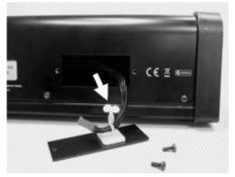
Insert the connector into the pins in the direction shown. Make sure that the references are on top. →
