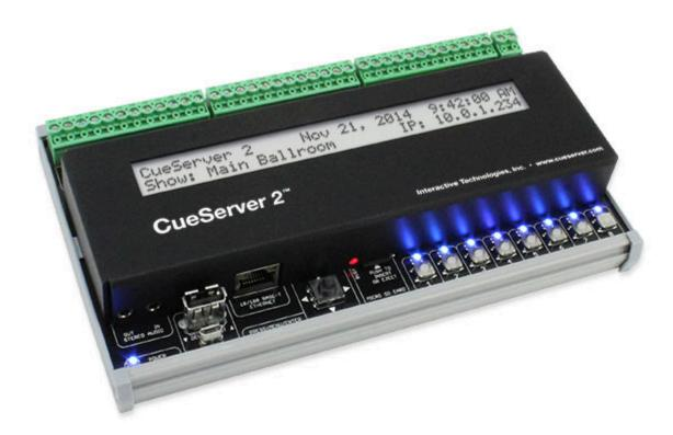
The CueServer 2 DIN is housed in an enclosure with replaceable side brackets suitable for DIN-Rail or surface mounting. It features a single LAN port, two DMX input ports, two DMX output ports, and eight user definable pushbutton inputs. See the <a href="CS-940 CueServer 2 DIN">CS-940 CueServer 2 DIN</a> section for more details for this model.
