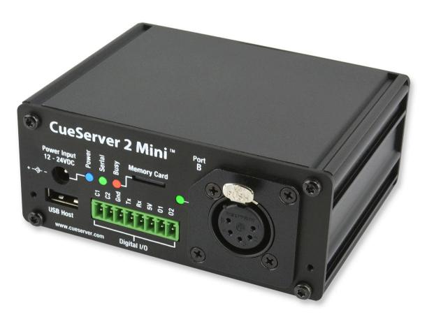
The CueServer 2 Mini is housed in a small enclosure suitable for desktop use. Optional brackets allow the CS-920 to be DIN Rail mounted, or attached to a flat surface, or hung from truss. It features a single LAN port, two field-replaceable DMX module slots, and two user definable pushbutton inputs. See the <a href="#">CS-920</a> <a href="#">CueServer 2 Mini</a> section for more details for this model.
