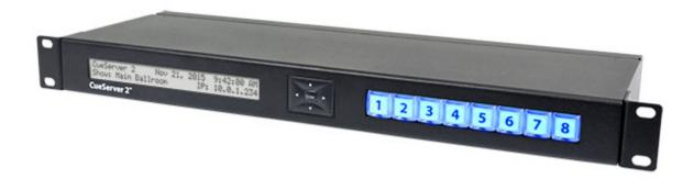
The CueServer 2 Pro is housed in an enclosure with removable brackets suitable for either 19" rack-mounting or desktop use. It features dual LAN ports, four field-replaceable DMX module slots, and eight user definable pushbutton inputs with customizable front-panel button caps. See the <a href="#">CS-900 CueServer 2</a> Pro section for more details for this model.
